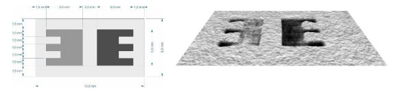
Figure 1: Test Patch Definition Figure 2: Scanning Image of Test Patch
